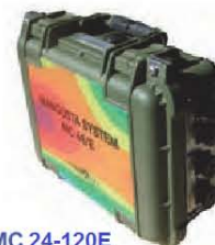
Mangusta MC 24-120E Geoelectrical Tomography Equipment
